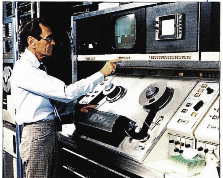
Two TR-22 VTRs that went on-air with Corpus Christi station in 1964 are still being used on daily basis.
